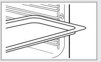
Wire shelf, Baking tray / Deep pan: Push the tray between the guide bars of the shelf support and the wire shelf on the guide bars above.
