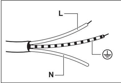
1. Connect the green and yellow (earth) wire to the terminal which is marked with the letter 'E', or the earth symbol
