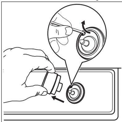
4. With a thin screwdriver, adjust the bypass screw position (A).
